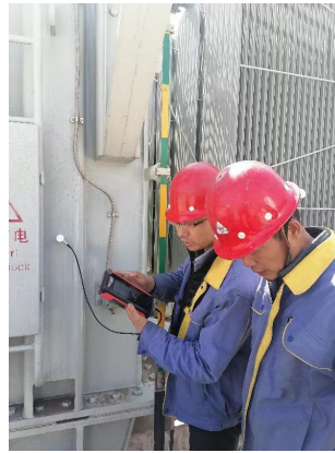
Test diagram of an external ultrasonic sensor
